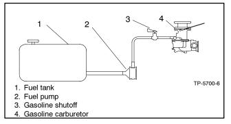
Figure 6-4 Gasoline Fuel System
